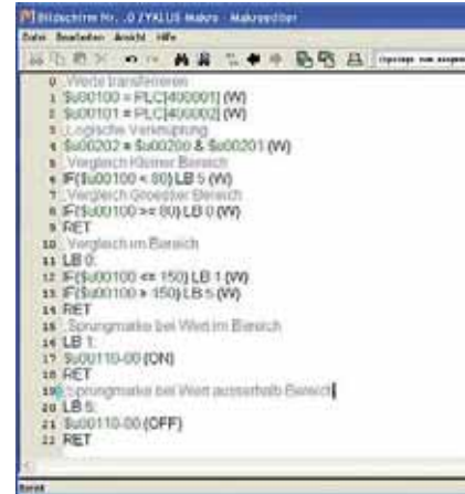
Easy to do: programming of basic PLC functions using the macro commands of the V-SFT programming software.
