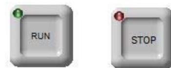
This is because the pressure drop has always priority and would connect the RUN command. To avoid it press STOP again. The system will then remain still till the RUN button is pressed again.
