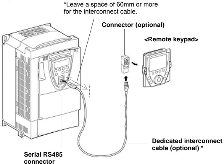
\*The pin configuration of the dedicated interconnect cable is different from that of any other commercially available cable. Therefore, be sure to use the dedicated interconnect cable.
