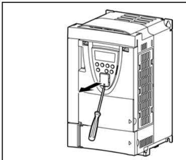
**2 Mount the remote keypad on the inverter's main operation panel.**
