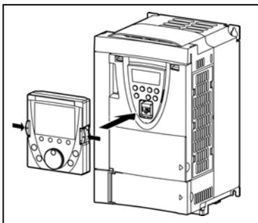
**3 Make sure the remote keypad is fixed securely to the inverter.**
