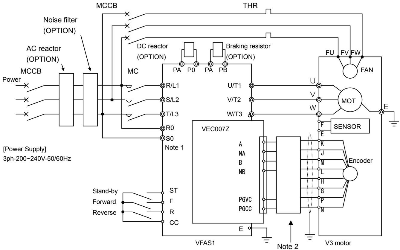
Note1 To divide the wiring between main power and control power, it is necessary to install CPS002Z(Backup unit of control power supply).
