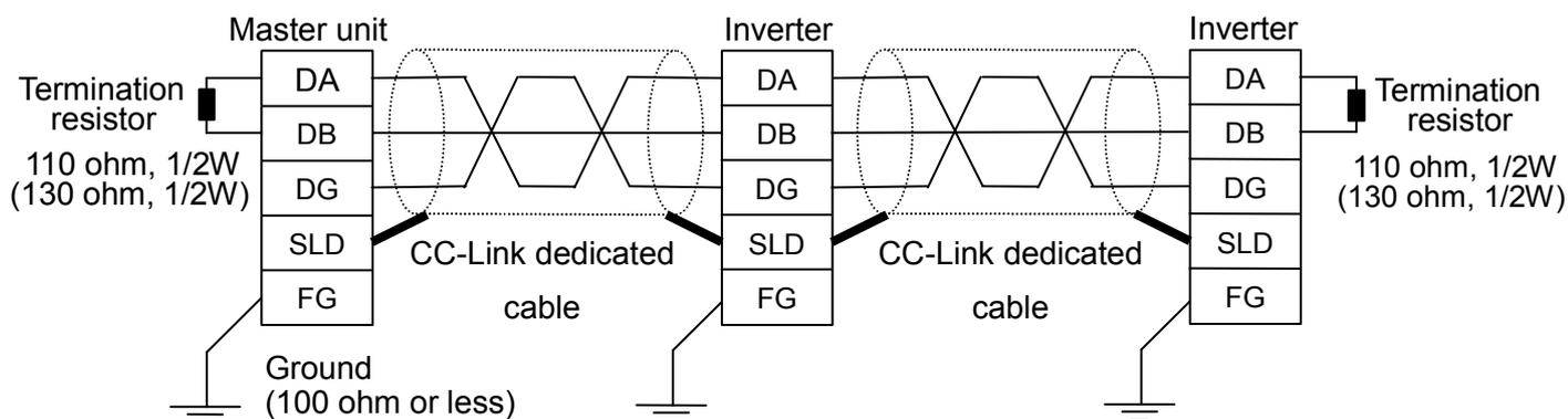
\* Maximum number of units connected to one master station is 42 units (when only inverters are connected).
