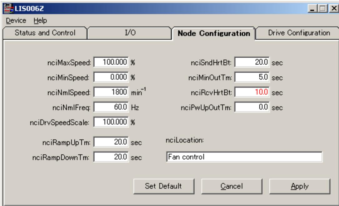
Input the configuration property text from keyboard. Changed value shows red text, it is not transmitted to the node yet. The functions of buttons are shown in the table below.
