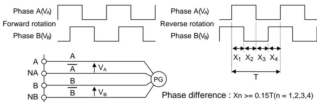
Figure 4-1 Judgement on normal and reverse rotations by the PG feedback of two phases (Phases A and B)
