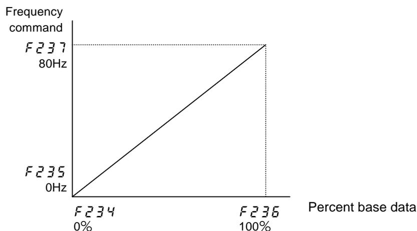
Figure 4-7 Percent base data and frequency command value
