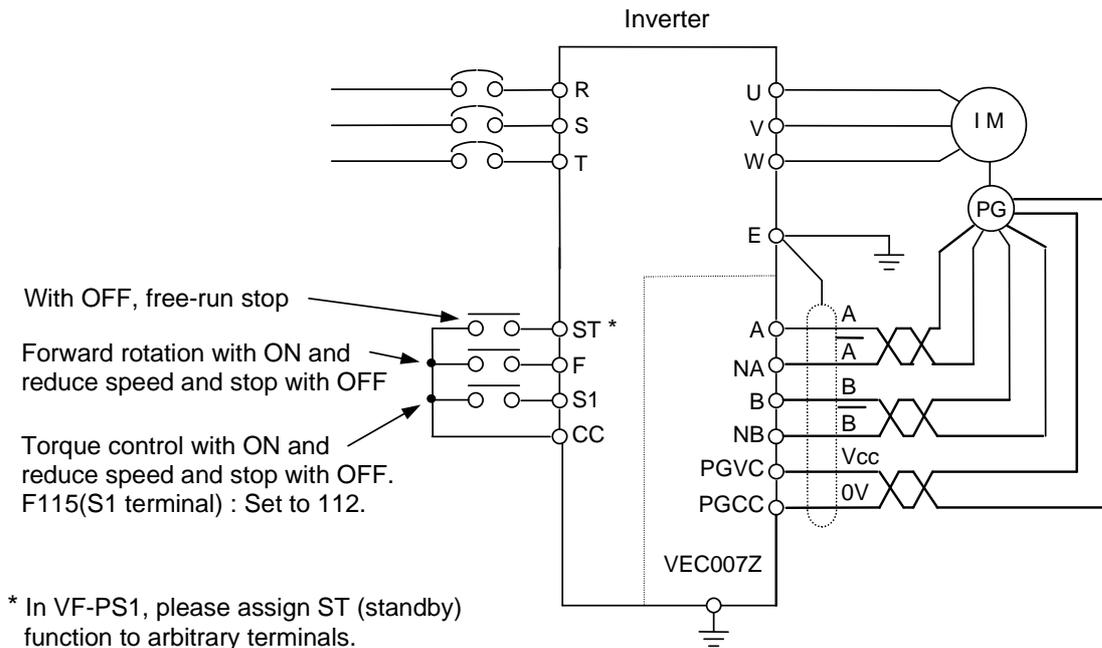
Figure 4-4 Example of wiring for line driver encoder (Speed/Torque switching operation)
