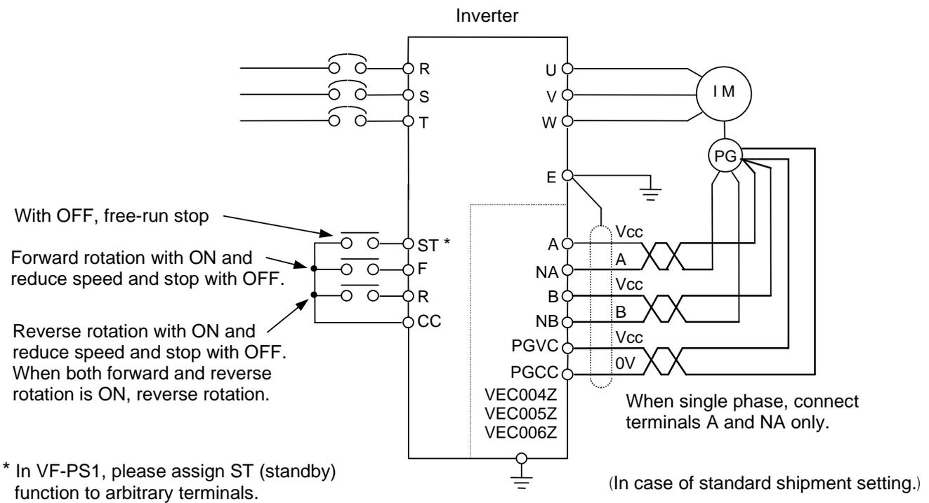
Figure 4-3 Example of open collector encoder connection
