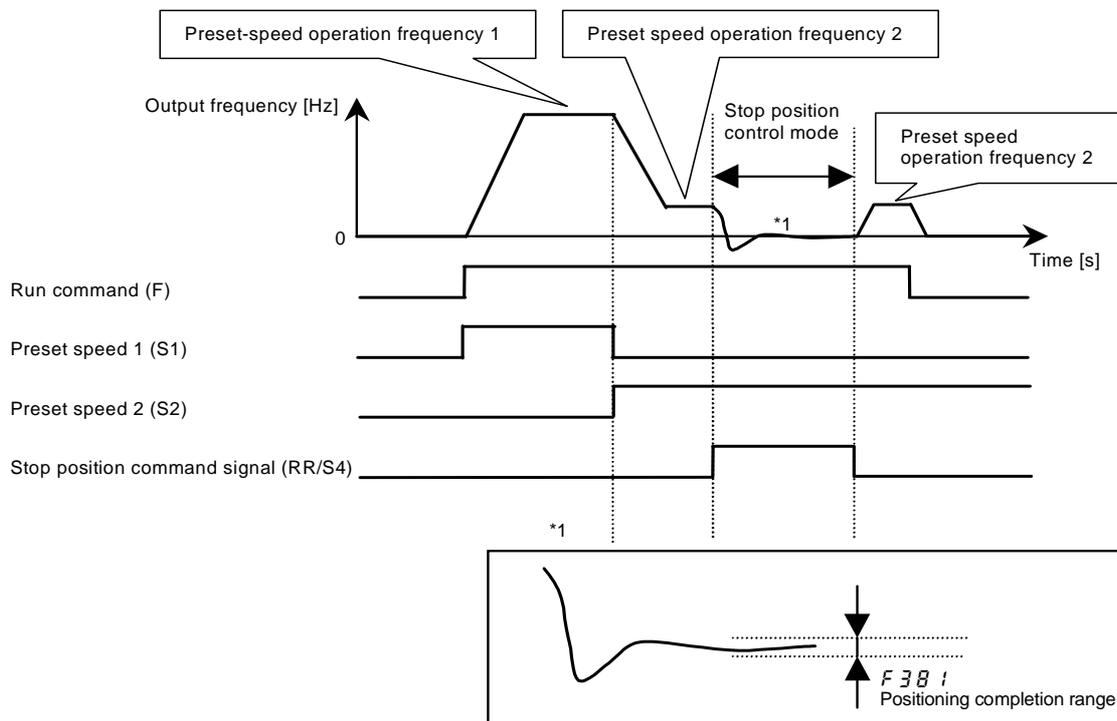
If the stop position control command is entered during high-speed operation, a trip may occur because of overcurrent or overvoltage. To avoid this, do not enter the stop position control command before the motor enters into low-speed operation.
