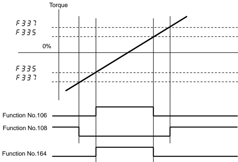
2) *F328* (Light-load high-speed operation selection) setting is not 0
