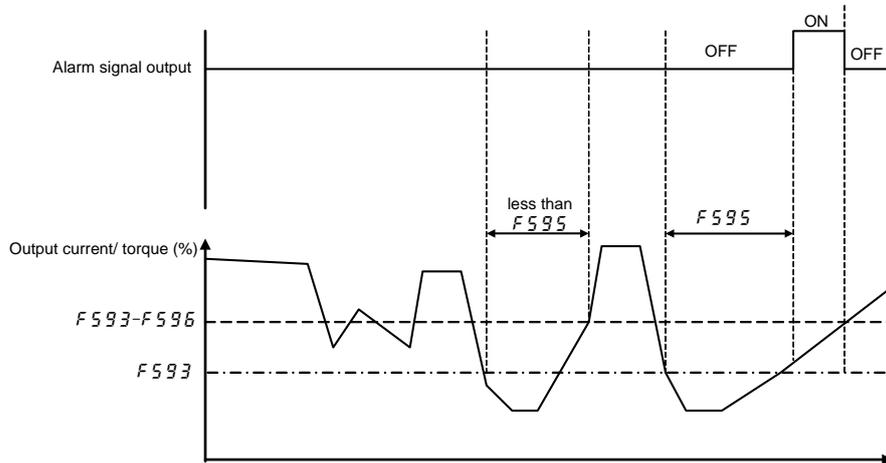
When setting  $F591=1$  (Tripping), inverter trips after low-current/ torque is detected for the period of time set with  $F595$ . Then, alarm signal remains ON.
