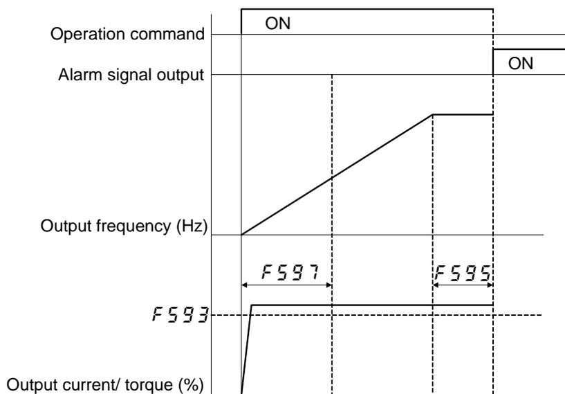
\* In case of less than  $F595$ , and the inverter is in acceleration/ deceleration status or over-current stall during detection activates, detection time will be reset.
