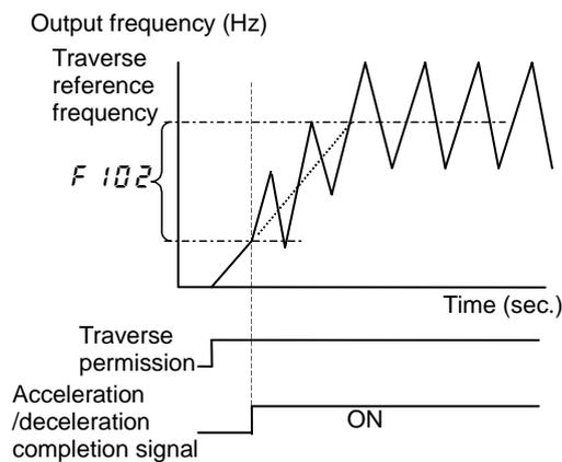
Fig. 3: Acceleration/deceleration completed with F 102 setting.
