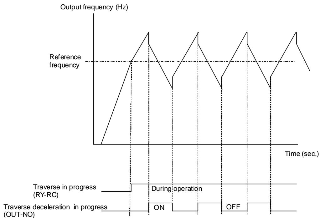
Fig. 5 Traverse output signals
