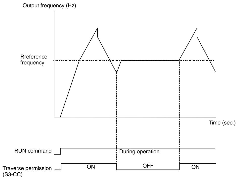
Fig. 4 Timing when the traverse function is off
