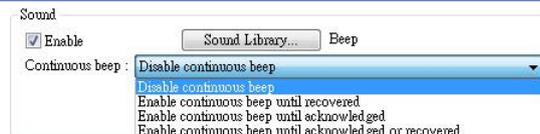
If enabled, the selected sound will be played when an event is triggered. Continuous beep can also be enabled, which only stops when the event is acknowledged or recovered.
