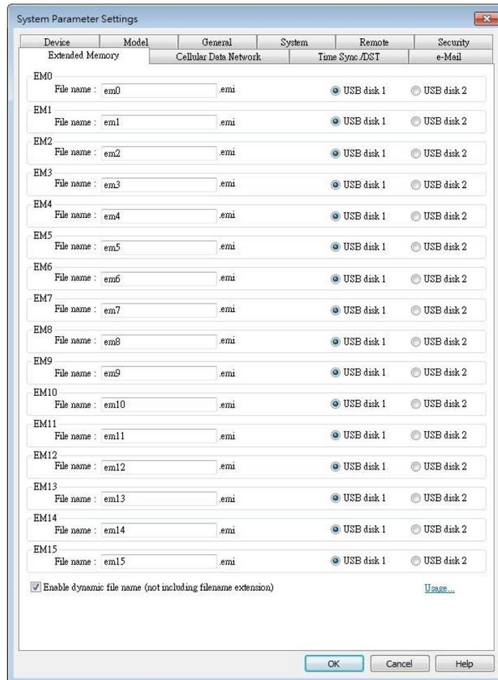
Extended Memory is numbered from EM0 to EM15. It works in a way similar to other device types (i.e. LW or RW address). Users can simply select from EM0 to EM15 in the [Address] setting while creating a new object. Maximum allowable data size for each Extended Memory is 2G words.
