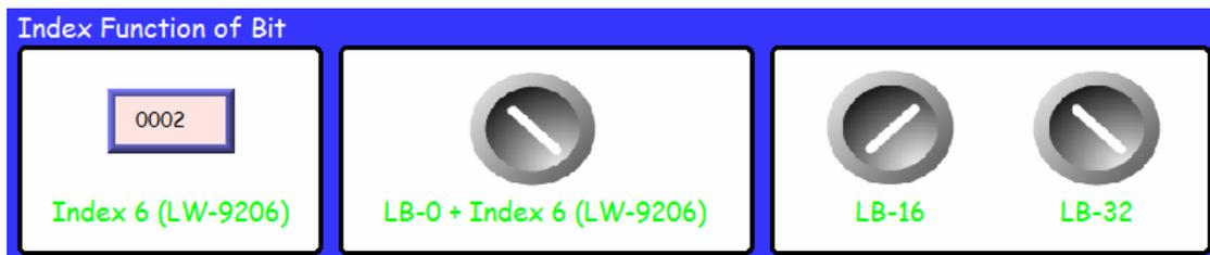
If Index 6 (LW-9206) is set to 2, then switch [LB-0 + Index6] reads LB-32 which is in OFF state.
