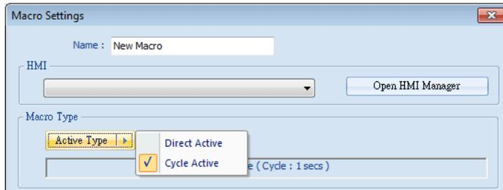
For example, if [Cycle Active] is set to 5 seconds, when executing a macro, the next time to execute the macro object will be 5 seconds later.
