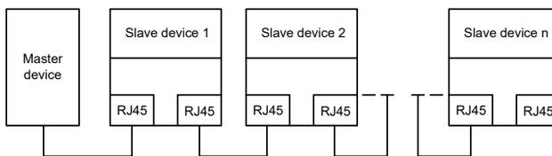
Linear network topology electrical connection diagram
