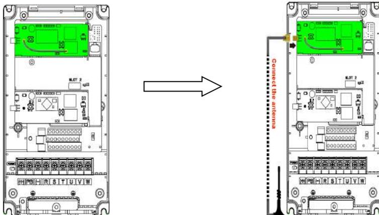
The wireless communication card must be used with the INVT VFD APP. Scan the QR code of the VFD nameplate to download it. For details, refer to the wireless communication card manual provided with the expansion card. The main interface is shown as follows.
