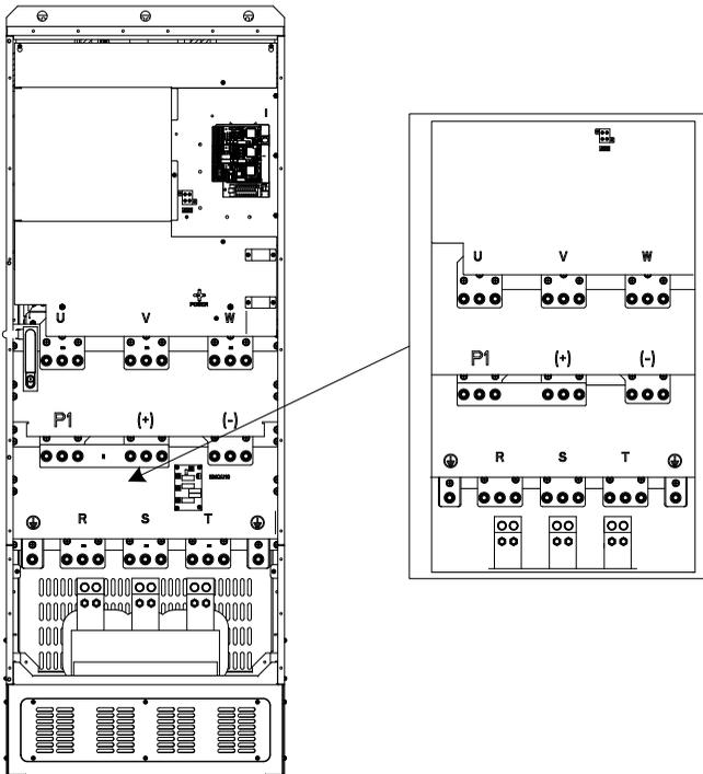
Figure 4.13 Main circuit terminal diagram for 355G/400P–500G models
