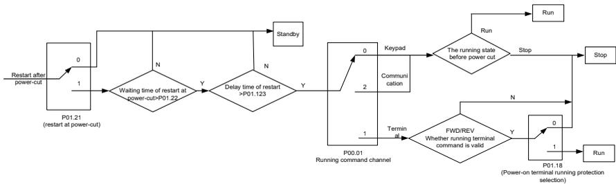
(3) Logic diagram for start after automatic fault reset
