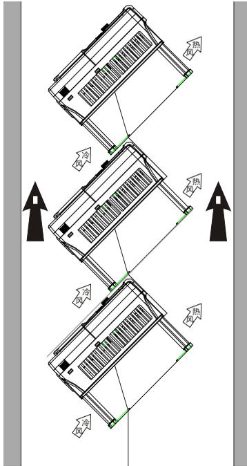
Figure 4.6 Tilted installation
