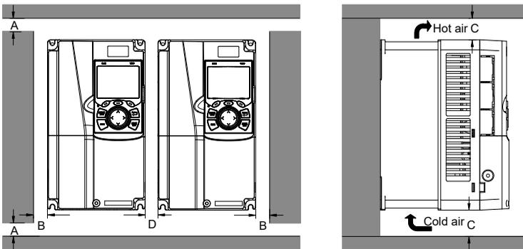
Figure 4.4 Parallel installation
