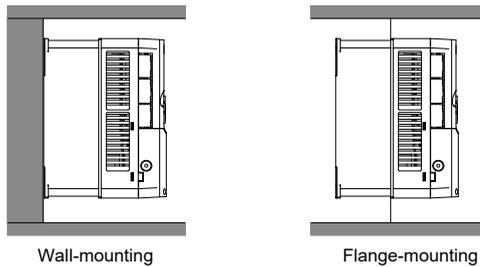
Figure 4.2 Installation mode
