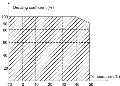
**Note:** It is not recommended to use the VFD at a temperature higher than 50°C. If you do, you shall be held accountable for the consequences caused.
