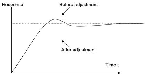
**Control short-term vibration:** If the vibration cycle is short is almost the same with the set value of derivative time ( $T_d$ ), it indicates derivative action is too strong, shorten the derivative time ( $T_d$ ) to control vibration. When derivative time ( $T_d$ ) is set to 0.00 (namely no derivative control), and there is no way to control vibration, decrease the proportional gain.
