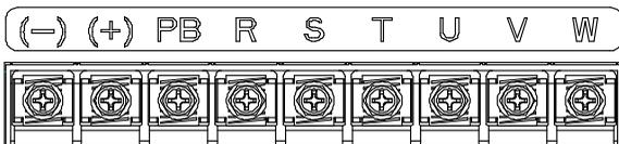
Figure 4.9 Main circuit terminal diagram for 030G/037P-037G/045P models
