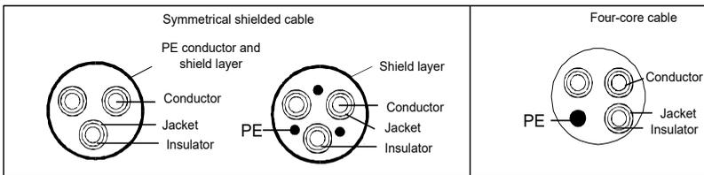
**Note:** If the conductivity of the shield layer of the motor cables cannot meet the requirements, separate PE conductors must be used.
