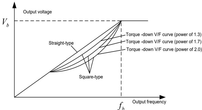
The VFD also provides multi-point V/F curves. You can change the V/F curves output by the VFD by setting the voltage and frequency of the three points in the middle. A whole curve consists of five points starting from (0Hz, 0V) and ending at (motor fundamental frequency, motor rated voltage). During setting, follow the rule:  $0 \leq f_1 \leq f_2 \leq f_3 \leq$  Motor fundamental frequency, and,  $0 \leq V_1 \leq V_2 \leq V_3 \leq$  Motor rated voltage
