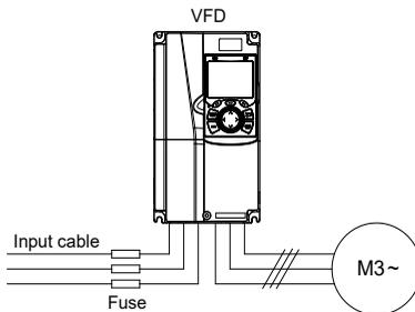
Figure 4.19 Fuse configuration
