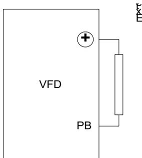
Installation of braking units:
