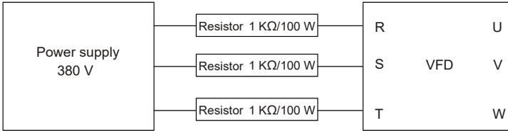
Figure 8.2 Charging circuit example of driving devices
