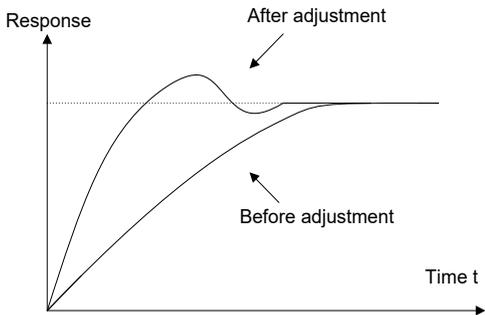
**Control long-term vibration:** If the cycle of periodic vibration is longer than the set value of integral time ( $T_i$ ), it indicates the integral action is too strong, prolong the integral time ( $T_i$ ) to control vibration.
