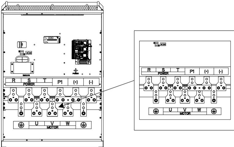
Figure 4.12 Main circuit terminal diagram for 220G/250P–315G/355P models
